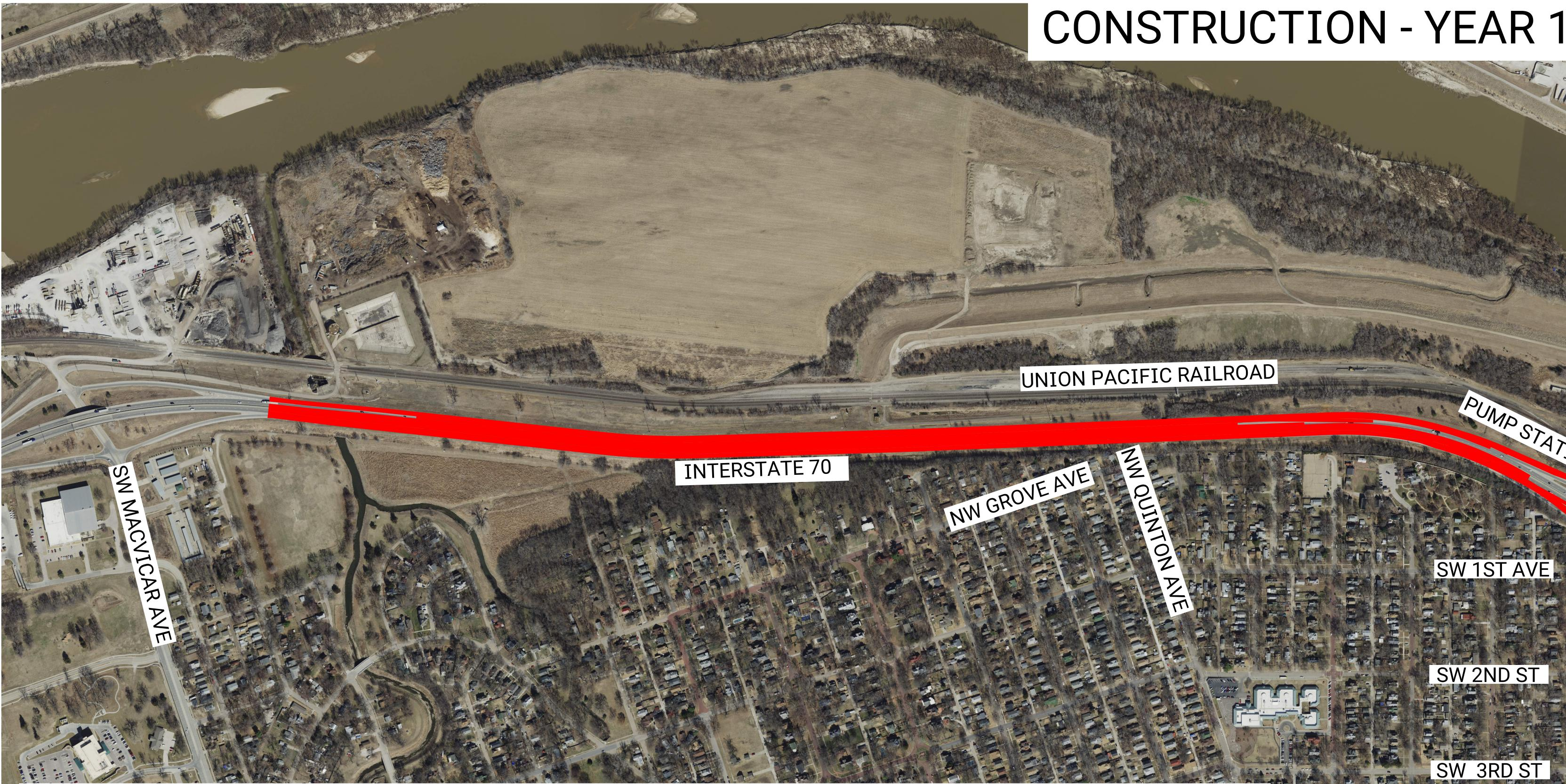
In the first year of construction, the new viaduct will be constructed offline while I-70 west to MacVicar Avenue will be widened. I-70 traffic will remain open during this year of construction. EB I-70 will be able to access Downtown Topeka via 1st St. and 3rd St. exits.
